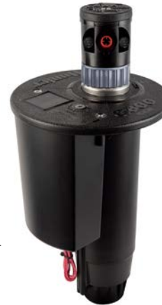
G-884E Pop-up height: 3¾" Overall height: 11¾" Flange diameter: 7¼" Female inlet: 1½" Acme
